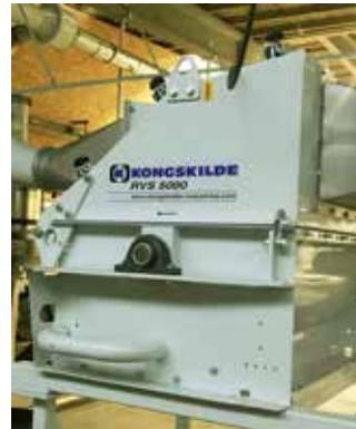
The RVS H Separator separates light material from the suction line air stream. The pipe connection on the side keeps the bearing area completely dust free.
